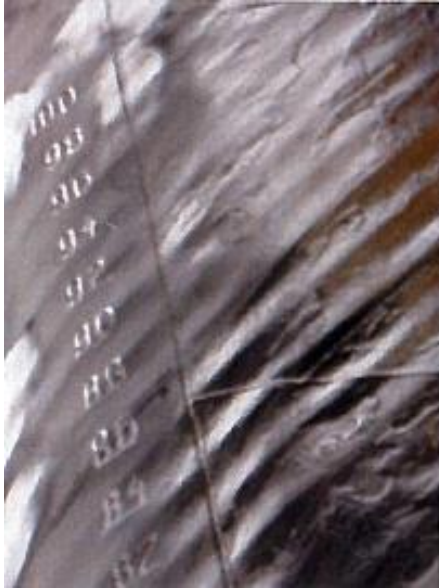
Damage of a chemical tanker's plating caused by multi-year ice (Hanninen, 2005)
